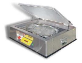
Clean room compatible machine, stainless steel chamber, designed to package trays, tubes, tape and reels. The use of a compressed air-driven vacuum pump minimizes noise, vibration and heat generation. Very accurate adjustment of vacuum which is controlled by an internal sensor.
