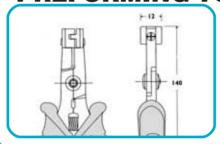
Professional tool specially designed to preform with central lead out of 3.81mm.
