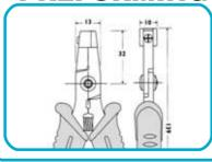
Professional tool specially designed to preform components at 90°.
