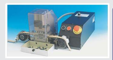
The AS1 is an automatic system that fits only the TP/R-PR machine. This equipment allows the machine to reach higher production. The driving wheel moves step by step stopping the tape during the preforming operation. It can be supplied to adapt the two most common hole pitches on the component tape: 12,7 (.5 inc.) (Code 95.OL11 for 110V, 95.OL12 for 220V) and 15 mm (.59 inc.) (Code 95.OL13 for 110V and 95.OL14 for 220V).
