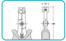
Professional tool specially designed to preform with central lead out of 3.81mm.
