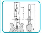
Professional tool specially designed to cut and preform components in a single operation. Variable length by means of an adjustable stop.
