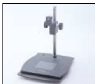
Camera stand (standard type) TW-CT1 A stand (with table) that holds the camera directly over the specimen and allows the camera to be inclined to the left or right. Dimensions : 250(width) x 320(height) x 300(depth) mm Weight: Approx. 2.6 kg
